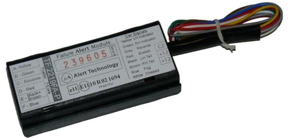
Upon power up, a full device self-check is automatically carried out and all relays exercised. Upon activating a lamp circuit, the Failure Alert Module provides a single Audible Alert signal (beep-beep) if a failed trailer bulb is detected.
